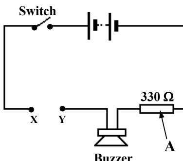
Name the component labelled **A** in the circuit. \_\_\_\_\_
