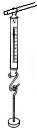
**Name** an instrument used to measure the force in this investigation.
